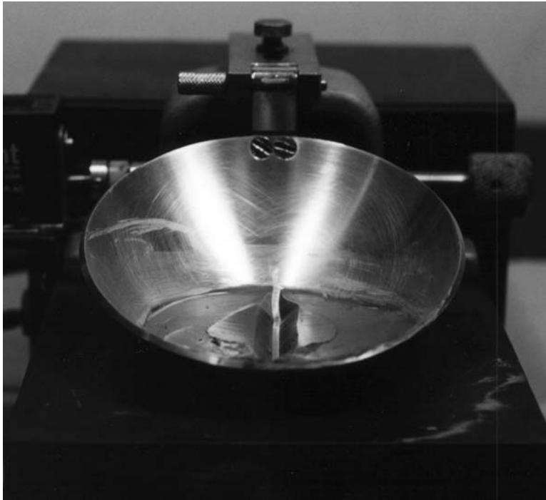
FIG. 7 Grooved Soil Pat in Liquid Limit Device
